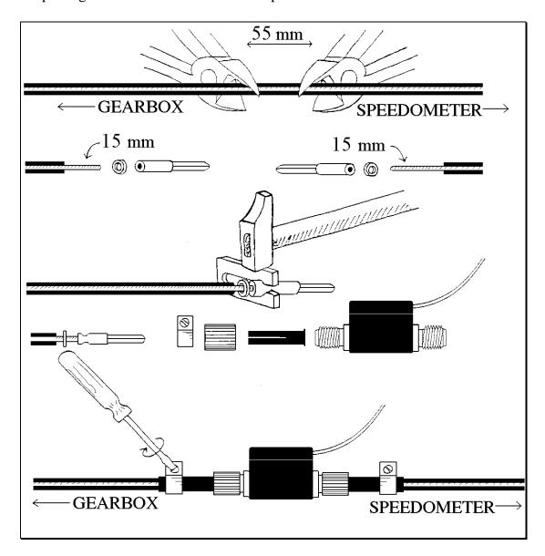
When removing the pulse generator from the vehicle you may replace it with a cable repair kit instead of changing the speedometer cable. The cable repair kit may be ordered from Jemba.
