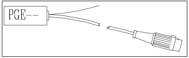
This interface is used in cars with electronic speedometer. It is connected to the original pulse generator of your car in accordance with a separate instruction.
