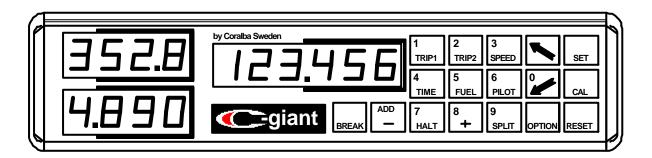
It is basically a distance- and speedo-meter for the car. Furthermore it has a lot of useful processing facilities for the co-driver. The precision of the instrument is reached by an effective but simple calibrating procedure. After calibration C-giant shows correct values to a tolerance typically better than 0.03%.
