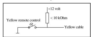
The yellow cable is meant to be connected to the reverse light as default. However you may define it as a remote control (See page 27). For this reason the remote control for the yellow cable should not be connected in the same way as for the white remote cable. It must
